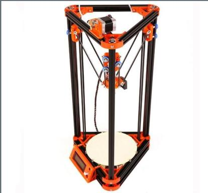
A team of four students are involved in the development of delta-type FDM 3D Printing machine for generation of printed components. Delta FDM printers uses a different system of movement for the printer nozzle. Instead of XYZ rods, delta printers support the extruder with three arms, which are attached to three vertical posts arranged in a triangle. Each arm can only move vertically up and down, but by moving each arm independently the extruder will be able to move in all directions.
